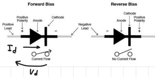
A diode is a semiconductor device that essentially acts as a one-way switch for current. It allows current to flow easily in one direction, but severely restricts current from flowing in the opposite direction.
