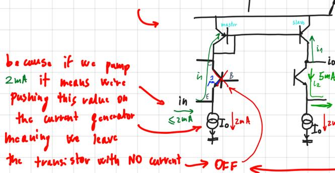
because if we pump 2mA it means we're pushing this value on the current generator meaning we leave the transistor with NO current  $\rightarrow$  OFF
