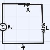
The inductor **DOESN'T** dissipate power → no voltage across the inductor
