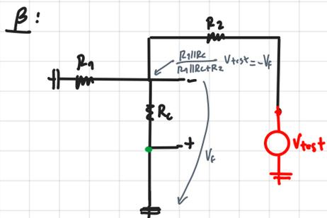
$$\beta = -\frac{R_1 \parallel R_c}{R_1 \parallel R_c + R_2}$$
