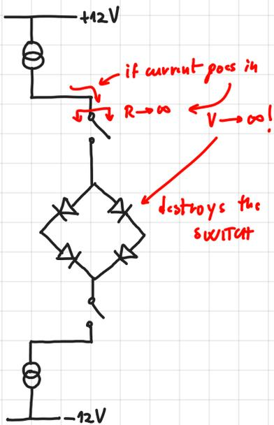
use instead differential pairs of pnp/npn transistors
