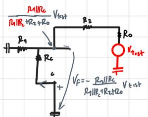
$$\beta = \frac{V_f}{V_{test}} = -\frac{R_1 \parallel R_c}{(R_1 \parallel R_c) + R_2 + R_o}$$
