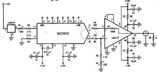
FIGURE 7. Fast Current-to-Voltage Current Mode DAC Amplifier
