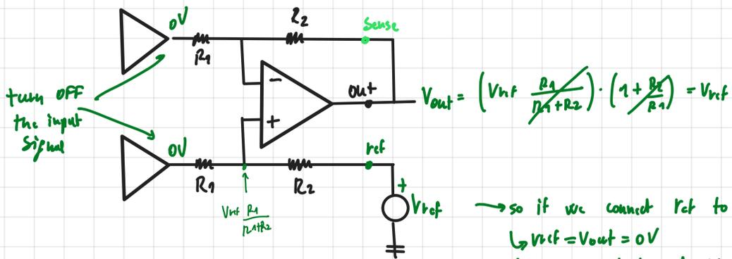
↳ so if we connect ref to ground  $V_{ref} = V_{out} = 0V$  (so it indeed act like a reference)
