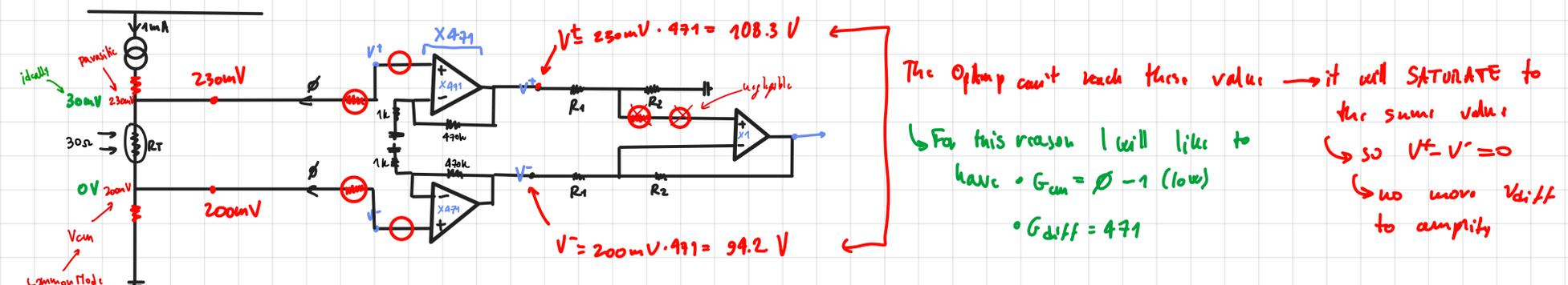
→ To amplify only the diff. signal and not the common mode a solution might be:
