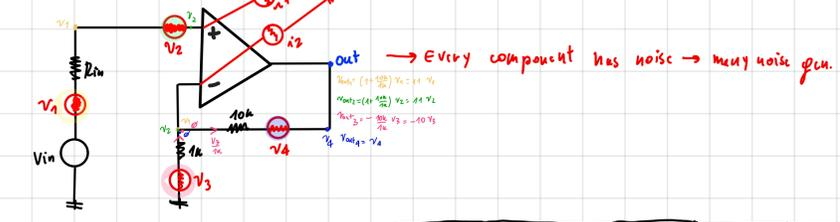
$$B.W. = 1MHz \rightarrow \sigma_{out} = rms_{out} = \sqrt{(v_1 \cdot 11 \cdot \sqrt{\frac{\pi}{2} 1MHz})^2 + (i_1 \cdot 11 \cdot \sqrt{\frac{\pi}{2} 1MHz})^2 + (v_2 \cdot 10 \cdot \sqrt{\frac{\pi}{2} 1MHz})^2 + (v_3 \cdot \sqrt{\frac{\pi}{2} 1MHz})^2}$$
