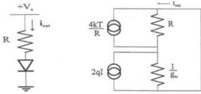
Fig. 1.19: Computation of the current noise in a biased junction (left) and an equivalent circuit for small signals (right) with the noise generators.
