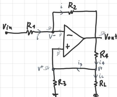
$$\frac{V_{in} - V^-}{R_1} = i = -\frac{V_{out} - V^-}{R_2} \quad (1)$$
