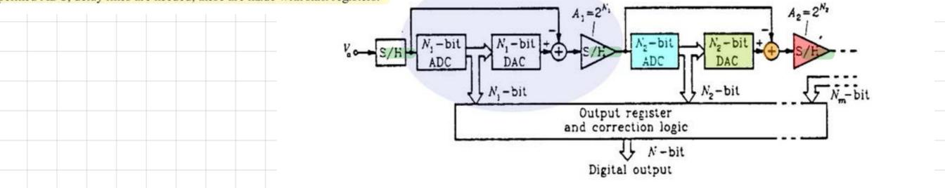
$m$ -stages each one composed by: ADC Flash (low resolution 1+4bit), DAC, analog adder and amplifying S&H
