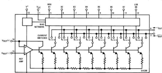
**Components:** •  $\sim 2n$  resistors → to provide  $\bar{I}_{out}$ ,  $I_{out}$
