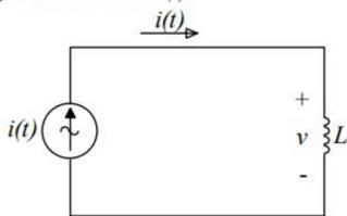
Figure 13. Fundamental inductor circuit
