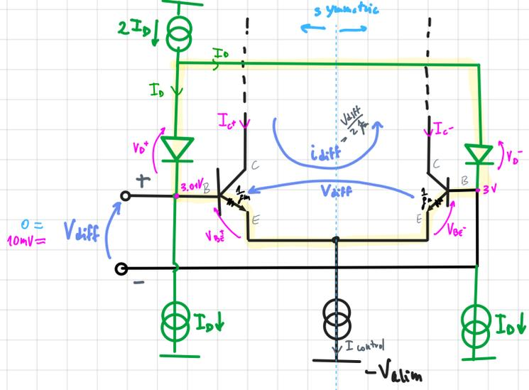
Case 1: The stage is fully symmetric ( $V_{diff}=0$ )
