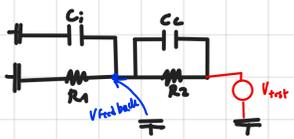
If  $R_1 C_i = R_2 C_c \rightarrow \frac{C_i}{C_c} = \frac{R_2}{R_1}$  the circuit is said to be **COMPENSATED**
