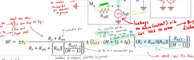
$$\Delta V = \pm v_s \cdot \frac{R_s + R_{on}}{R_s + R_{on} + \left[ R_{in} \parallel \left( \frac{R_{off}}{M-1} \right) \right]} \pm (I_{off} \cdot (M+1) + I_b) \cdot \left\{ (R_s + R_{on}) \parallel \left[ \frac{R_{off}}{M-1} \right] \right\}$$
