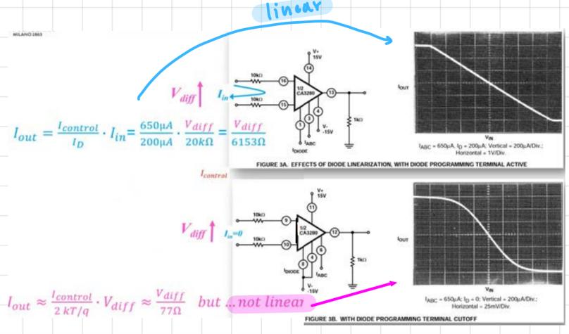
$$I_{out} \approx \frac{I_{control}}{2kT/q} \cdot V_{diff} \approx \frac{V_{diff}}{77\Omega} \text{ but } \dots \text{ not linear}$$
