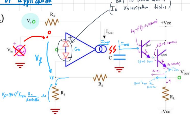
A secondary effect of the differential stage is that when we increase  $I_{control}$  the pole increases, this is due to the parasitic capacitances inside the OTA amplifier.
