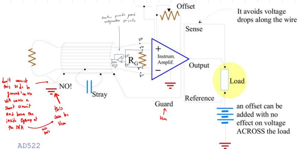
don't connect this side to ground! cause will cause a short circuit and burn the inside OpAmp of the INA. use this. this can be  $V_{cm}$
