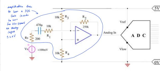
amplification does to have a X25 Gain in order to have for Vin=500mV an output input  $\pm 2.5V$
