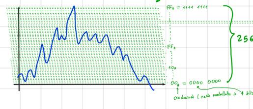
smallest level an ADC can convert
