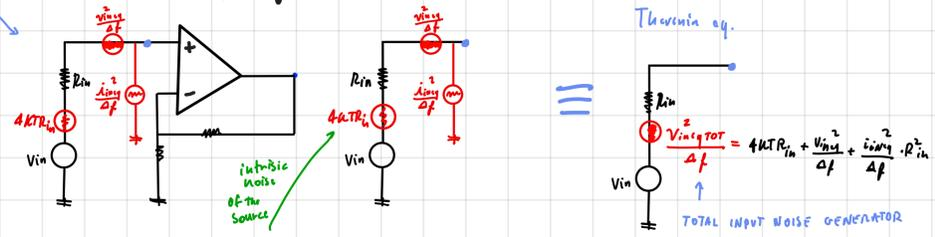
$$V_{noise, total}^2 = 4kTR_{in} \Delta f + \frac{v_n^2}{\Delta f} + \frac{i_n^2 \cdot R_{in}^2}{\Delta f}$$
