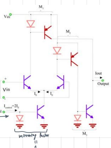
$$g_m = \frac{dI_{OUT}}{dV_{diff}} = \frac{dI_{OUT}}{d(V_+ - V_-)} = \frac{2I_E}{kT/q} = \frac{I_{control}/2}{kT/q}$$
