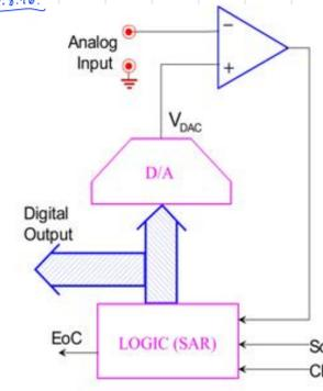
Components: 1 DAC and 1 sequential SAR logic
