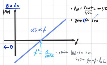
•  $A_v = \frac{V_{out}}{V_{in}} = -s\tau$
