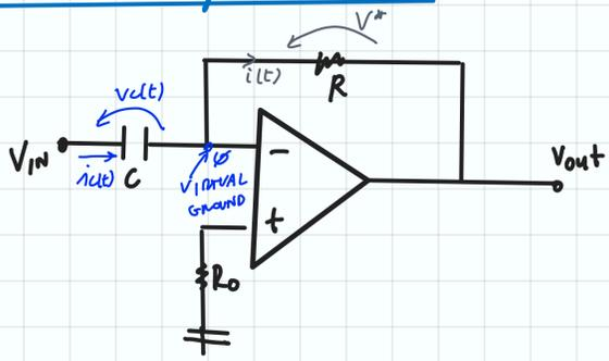
Capacitor  $i(t) = i_c(t) = C \frac{dV_c(t)}{dt} = C \frac{dV_{in}(t)}{dt}$
