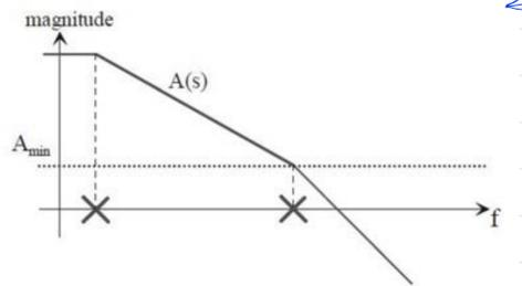
Fig. 3.73:  $A_{min}$  represents the minimum gain that can be used without needing any compensation.
