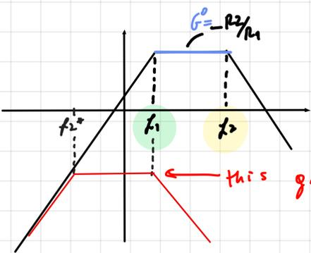
$\rightarrow$  if  $f_1 > f_2^*$  it means that the circuit with  $R_2, C_2$  switches to short circuit  $f > f_2 (< f_1)$  before the circuit  $R_1, C_1$  it will kill the signal before that circuit
