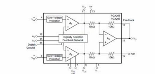
Many INAs are provided with some internal resistors to set the gain, simply shorting the pins to the ground. Some INAs have circuitry to protect the front-end Op-Amps from overvoltage. Furthermore, there are buffers that can be used as Guard Outputs, which are connected to the coaxial cable that brings the signal (Fig. 4.13).
