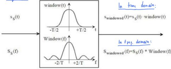
Fig. 6.27: Windowing effect on original sequence samples.
