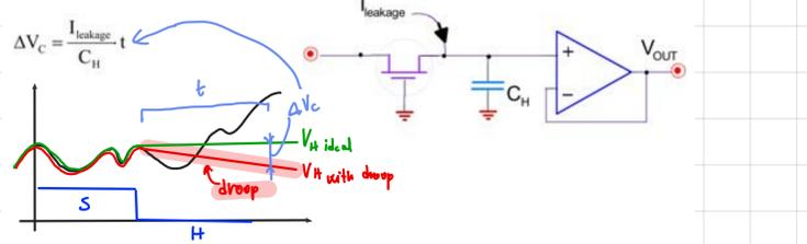
With  $I_{leakage} = 100pA$  and  $C_H = 9nF$ , the stored voltage will droop by 11mV/s
