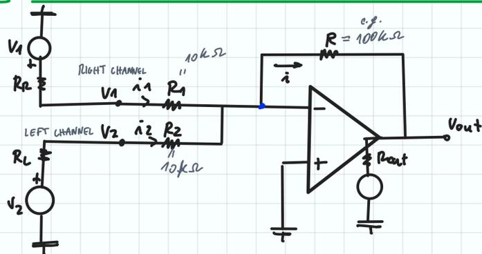
→ If we have  $R_1=R_2=10k\Omega$  → to have  $G_L=G_R = -\frac{R}{R_i} = -10$  but  $R_L \neq R_R$  it means
