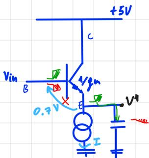
The capacitor is quickly charged by the transistor  $\rightarrow$  PULL-UP stage.
