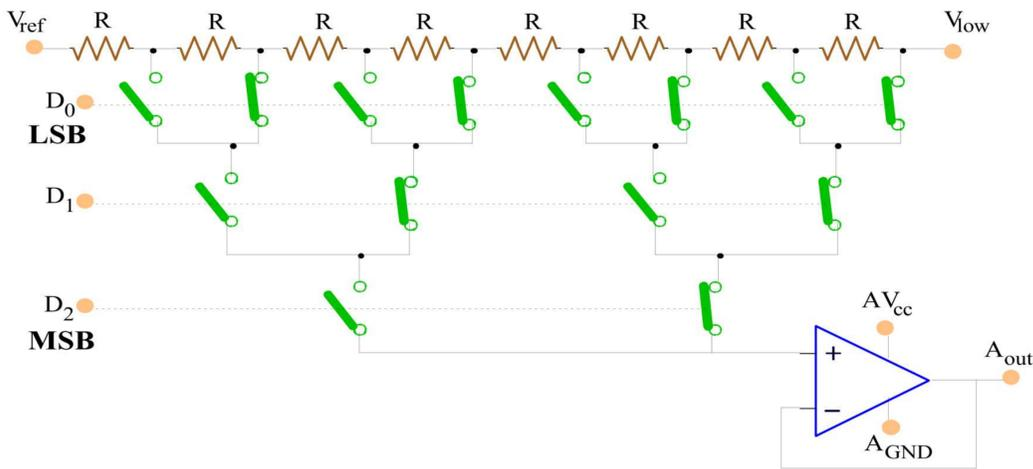
**Components:** •  $2^n$  Resistors → divide FS<sub>R</sub> in  $2^n$  voltage level
