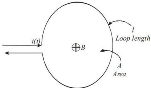
Figure 11. Current loop for the calculation of inductance
