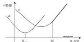
Fig. 1.15: Comparison between two different trends of NF as a function of  $R_s$ .
