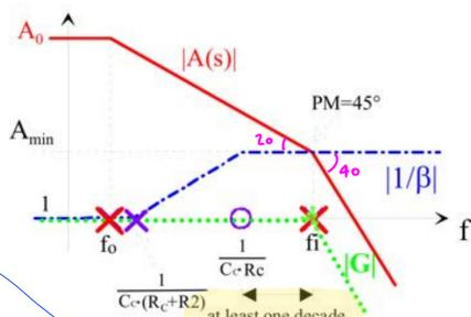
In the case of a high frequency buffer, the aforementioned compensation could not work. To solve this problem, we introduce a resistor  $R_2$  that provides positive feedback. In practice, it happens that in the magnitude Bode plots, the  $1/\beta$  starts to rise at lower frequencies. It is important to note that this is the only compensation method for voltage-followers. Let us consider the circuit in Fig. 3.77.
