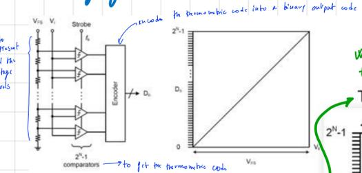
In standard Flash ADCs, comparators near  $V_{in}$  are important just for the "fine" conversion, hence they are useless for the "coarse" one, thus the architecture wastes resources and is not efficient
