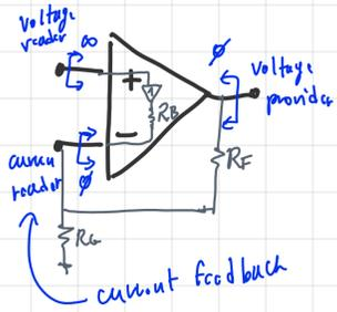
$$G_{CFA} = 1 + \frac{R_f}{R_g}$$
