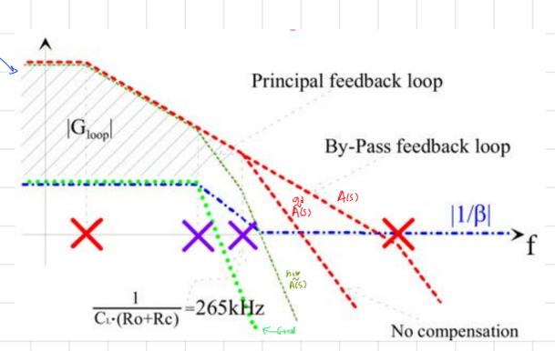
$$\frac{1}{C_L \cdot (R_0 + R_C)} = 265 \text{ kHz}$$
