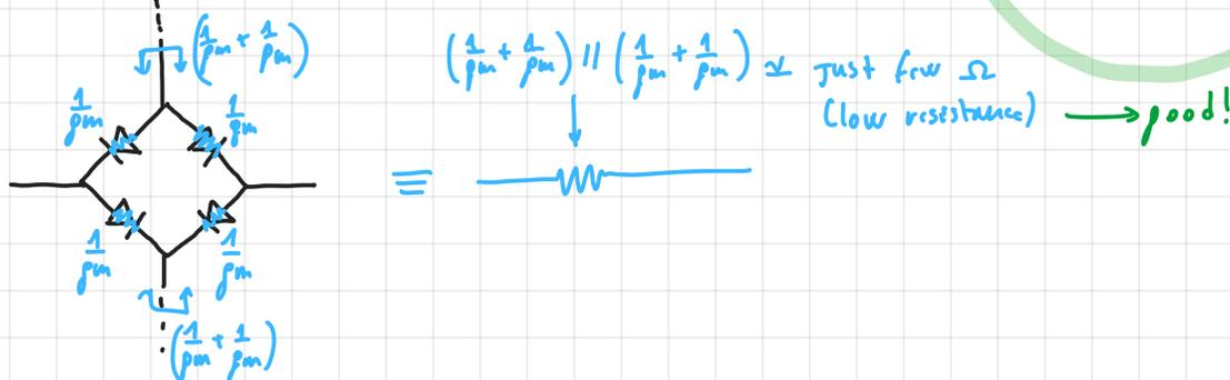
This switch presents a disadvantage in terms of feedthrough → indeed consider the case where the CH has a value smaller than the one of Vin → 2 diodes will be forward bias and 2 not.
