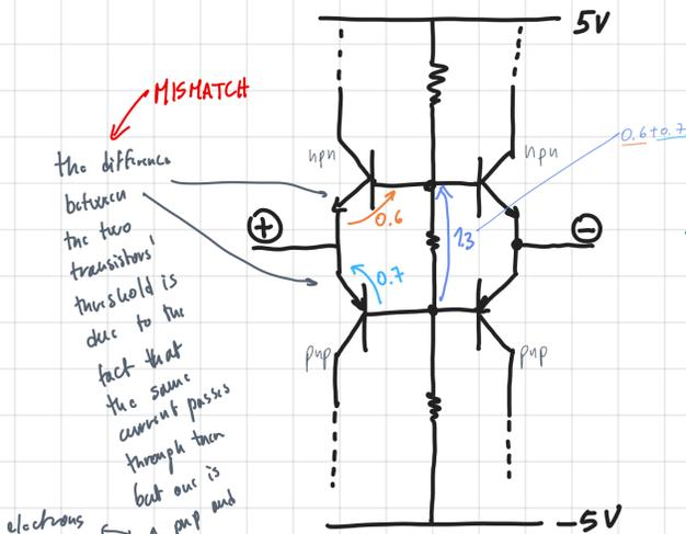
usually for the same dimension the voltage drop across an npn will be lower, 'cause the efficiency of the holes is worst w.r.t the electrons
