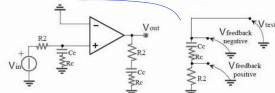
Observe that the input compensation network is bootstrapped and that the effect of loading the input node is then reduced. The input impedance is:
