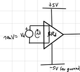
$$R_d = \frac{V_d}{i_d} = \frac{10mV}{1\mu A} = 10k\Omega$$
