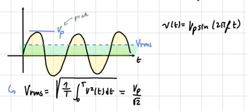
The power of  $v(t)$  is equal to the power of a DC Volt  $V_{rms}$
