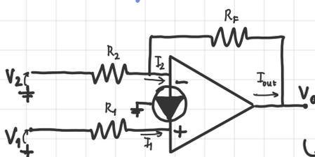
$$I_1 = \frac{V_1}{R_1} \quad I_2 = \frac{V_2}{R_2} \quad I_0 = \frac{V_0}{R_0}$$
