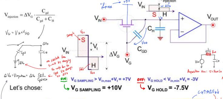
To guarantee  $V_{injection} \leq 1mV$  with  $\Delta V_G = \Delta V_{G,max} = 17.5V$  we chose  $C_H \geq 9nF$ ... hence the bandwidth is set to just 354kHz
