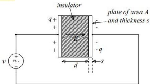
Figure 2. Capacitor model
