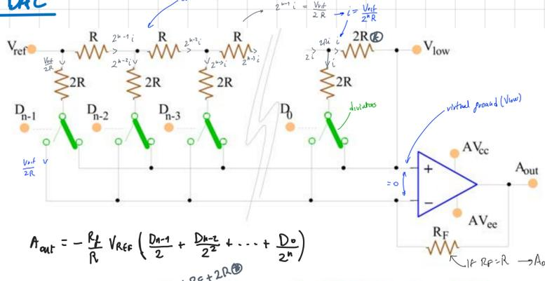
$$A_{out} = -\frac{R_f}{R} V_{REF} \left( \frac{D_{n-1}}{2} + \frac{D_{n-2}}{2^2} + \dots + \frac{D_0}{2^n} \right)$$
