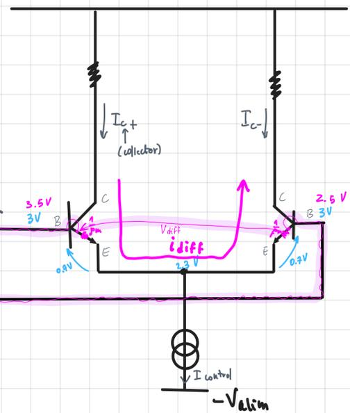
• Case 1:  $I_{control}$  splits in 2 →  $I_c = \frac{I_{control}}{2}$  ( $V_{diff} = 0$ )
