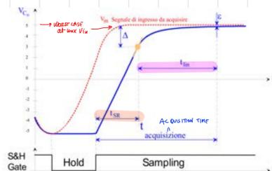
Acquisition (Sampling): linear ramp  $t_{SR} = \frac{10 - \Delta}{SR} = \frac{(10 - 1.25)V}{2.8V/\mu s} = 3.1\mu s$
