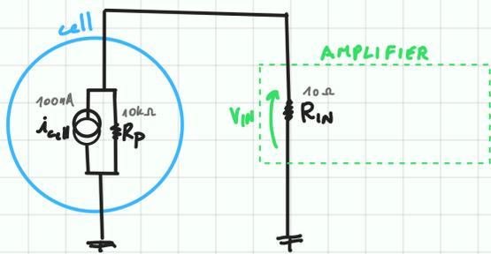
→ with  $R_{in} \ll R_p$  → almost no voltage drop
