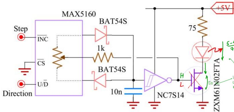
→ the LED will blink depending on the duty cycle of the oscillation
