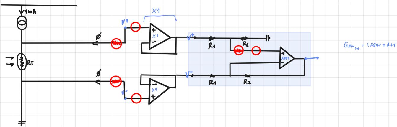
↳ Obs. If we put many stages in series is better to put the one with the higher stage before in this way only its noise contribution will affect the out-signal and the contributions of following stages with small noise will be negligible. If we instead put in series stages with small gain before the ones with higher gains all noise contributions will be collected going to the out signal.
