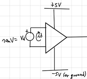
→ If we measure a differential current we can model  $R_{IN}$  as a differential impedance  $R_d$ :
