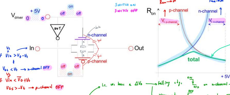
for the switches: just one transistor is not enough, because analog inputs can vary a lot b/w pos. and neg. values so to properly close the switch we shall use a transistor pair of p-channel and n-channel driven with opposite phases
