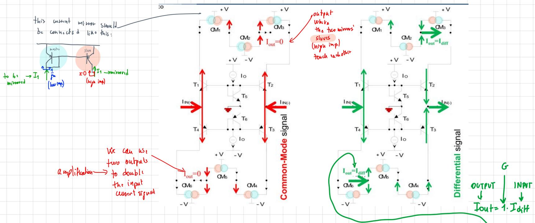
But how if we use this configuration the gain of the amplifier will be 1 at best, so if we want to increase the amplification we can use a current mirror that is not symmetric, meaning a mirror side amplifies the other:
