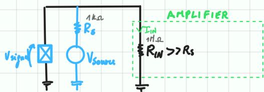
→ with  $R_{in} \gg R_s$  → almost no current flowing into  $R_{in}$  (or into the circuit)
