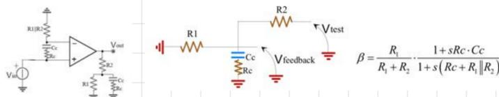
$$\beta = \frac{R_1}{R_1 + R_2} \cdot \frac{1 + sR_c \cdot C_c}{1 + s(R_c + R_1 \parallel R_2)}$$
