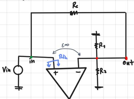
$$R_{in} = \frac{R_{stupid}}{1 - G_{loop}} = \frac{R_c + (R_1 \parallel R_2)}{1 - 1.1} \rightarrow \infty$$
