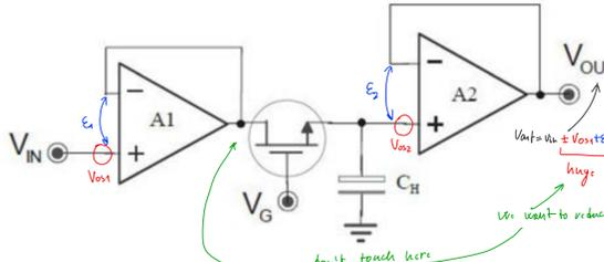
Fig. 6.43: S&H with an input buffer to improve the acquisition speed.
