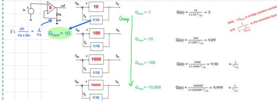
Note:  $1 - G_{loop}$  is a large positive number and  $\frac{1}{1 - G_{loop}}$  is the correction factor
