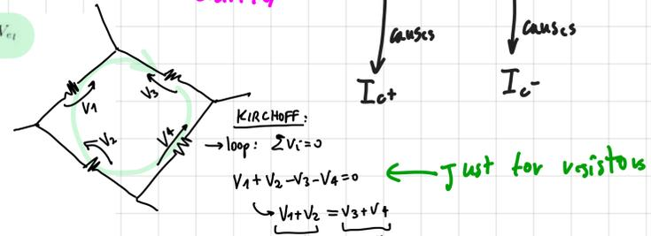
Every time we have a loop with diodes/transistors we can apply the translinear principle
