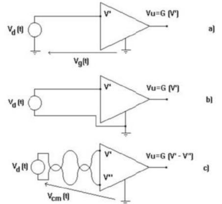
Fig. 1.5: Connection schemes of a sensor to an amplifier: a) single-ended through ground; b) single-ended through two wires; c) differential sensing.
