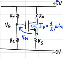
Operating conditions (for the MOSFET to work like an amplifier)
