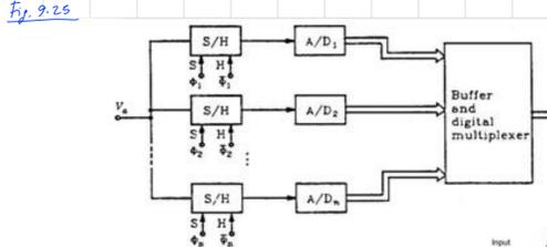
For high  $f_s$  more ADC can run in parallel on different samples:
