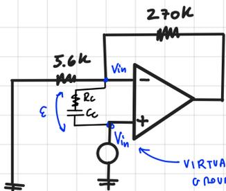
the components introduced don't change the gain (negative feedback) concept
