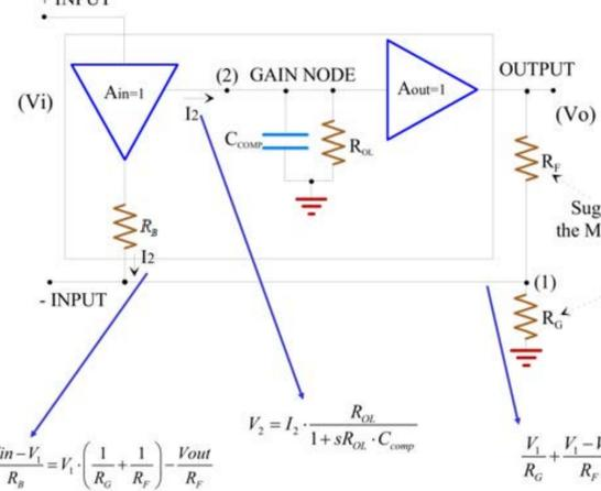
With open-loop:  $pole_{openloop} \approx \frac{-1}{C_{comp} \cdot R_{OL}}$   $G_{loop} \approx -R_{OL} \cdot A_{out} \cdot \frac{1}{R_B + R_F} \approx -\frac{R_{OL}}{R_F}$
