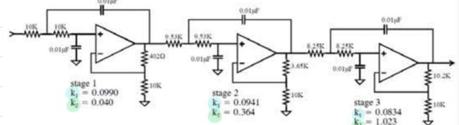
FIGURE 3-9 A six-pole Bessel filter formed by cascading three Sallen-Key circuits. This is a low-pass filter with a cutoff frequency of 1 kHz.
