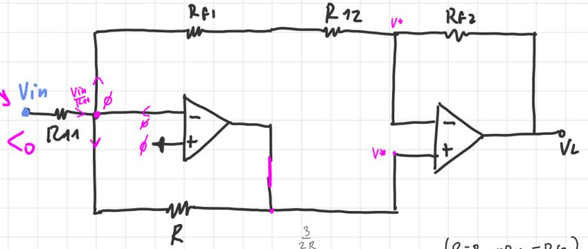
$$-\left(\frac{V^+}{R_{f1} + R_{f2}} + \frac{V^+}{R}\right) = \frac{V_{in}}{R_{f1}} \rightarrow V^+ \left(\frac{1}{R_{f1} + R_{f2}} + \frac{1}{R}\right) = -\frac{V_{in}}{R_{f1}} \rightarrow V^+ = -\frac{R}{R_{f1}} V_{in}$$
