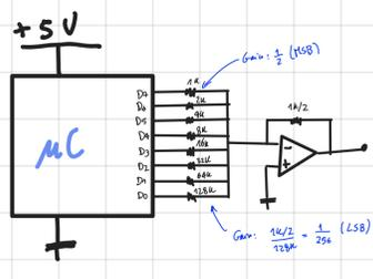
Due to the fact that the offset changes with  $D_{in}$  (due to MOS) in this type of config., because when switches are all open  $\rightarrow R_{eq} = \infty$ , when they're all close the resistors are all in parallel  $R_{eq} \approx \frac{R}{2} \rightarrow$  gain changes with  $D_{in}$
