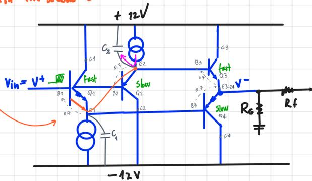
→ Now we QUICKLY pump current into that node letting  $E2$  quickly increase (vs increase also the SR)
