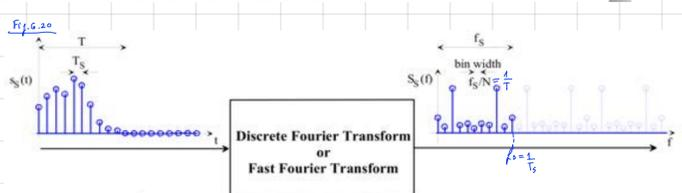
The FFT algorithm trusts on the periodicity of the input sequence ... hence FFT spectrum is for the periodic sequence and not the original one!
