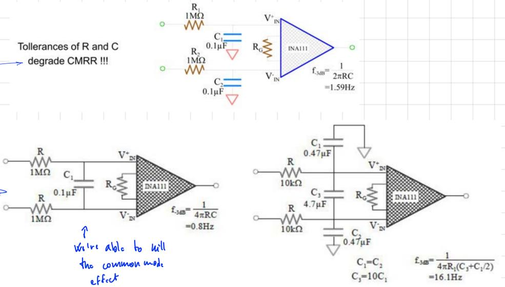
Fig. 4.8: Differential low-pass (on the left) and common mode (on the right) filtering.
