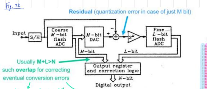
Conversion is a two-steps process through two cascaded stages. Such "half-flash" (or "two-step flash") approach drastically reduces: components count, power dissipation, input capacitance.
