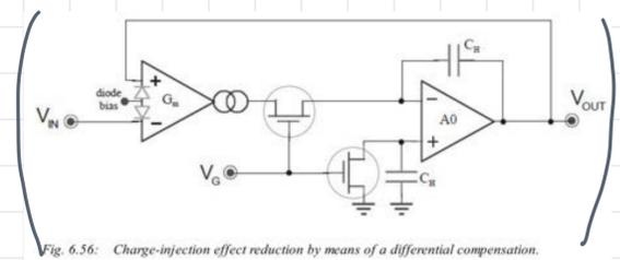
Fig. 6.56: Charge-injection effect reduction by means of a differential compensation.
