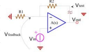
$$\beta = \frac{V_{feedback}}{V_{test}} = \frac{R_1}{R_1 + R_2}$$
