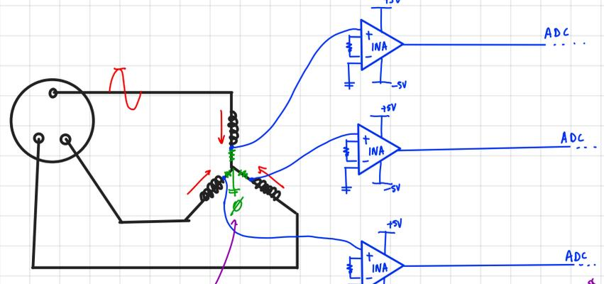
If this ground moves or disconnect (thin the signal will move again for  $\pm 542V$ ) -> destroy OpAmps and ADC.
