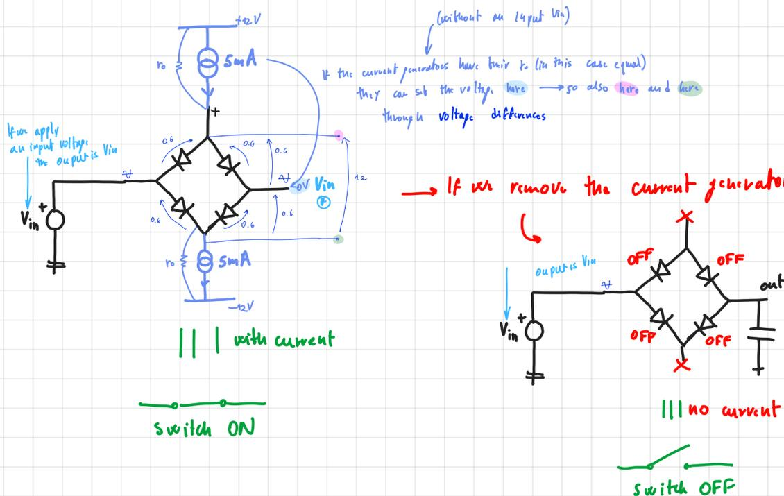
To control the current, so the bridge / switch ON and OFF modes, we can put another (different) switch between the current sources and the bridge:
