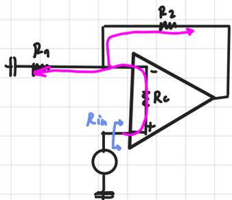
$$R_{in} = \frac{R_{stupid}}{1 - G_{loop}} = [R_c + (R_1 \parallel R_2)] + (1 + A_o \cdot \frac{R_1 \parallel R_c}{R_1 \parallel R_c + R_2})$$
