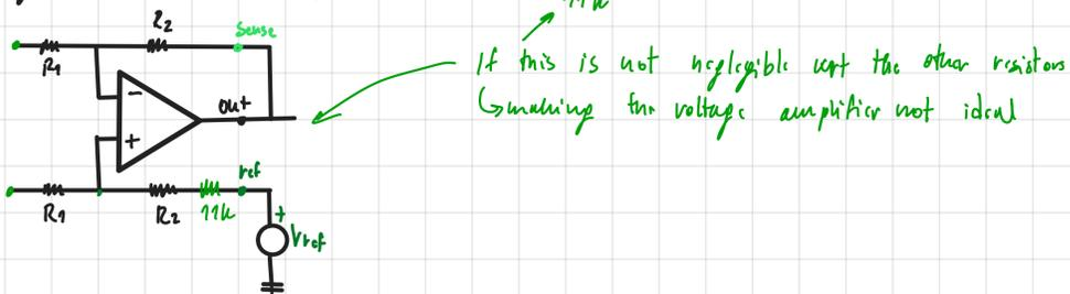
If this is not negligible w.r.t. the other resistors (making the voltage amplifier not ideal)
