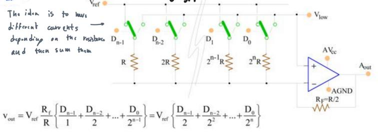
**Components:** n resistors (not quite...) and 2-n MOSFETs (p-MOS to  $V_{ref}$ , n-MOS to  $V_{low}$ )
