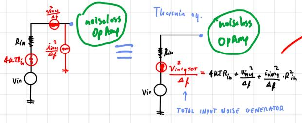
So now the resistor seems to be noisier than the intrinsic resistor because we also consider the noise of the OpAmp
