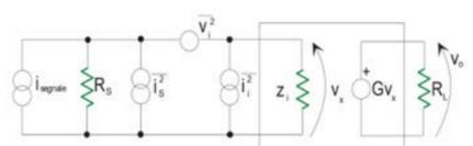
Fig. 1.14: Representation of the equivalent input noise, for the noise figure computation.
