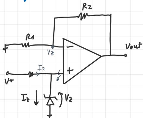
$$V_{out} = V_z \left( 1 + \frac{R_2}{R_1} \right)$$
