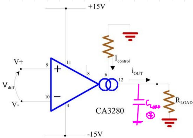
$$i_{out} = G_m(I_{control}) \cdot v_{diff} = \frac{I_{control}}{kT/q} \cdot v_{diff} = \frac{I_{control}}{25mV} \cdot v_{diff}$$
