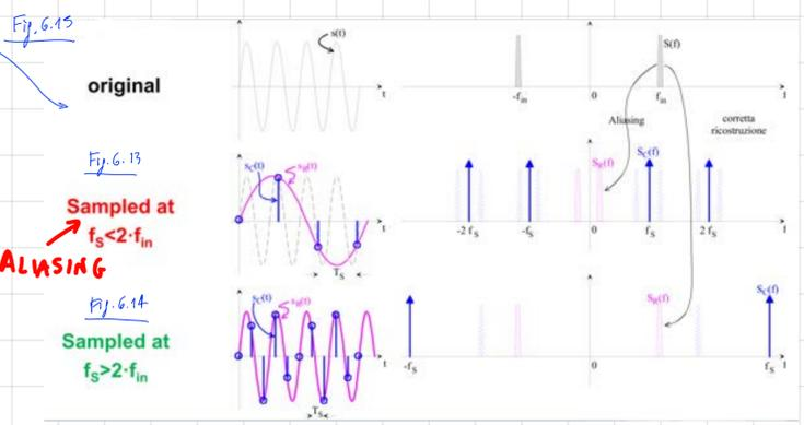
Aliasing stems out also from unexpected spurious disturbances with  $f_{\text{spur}} > f_s/2$
