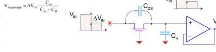
With  $\Delta V_{in,max} = 10V$  we get  $V_{injection} = 111\mu V$
