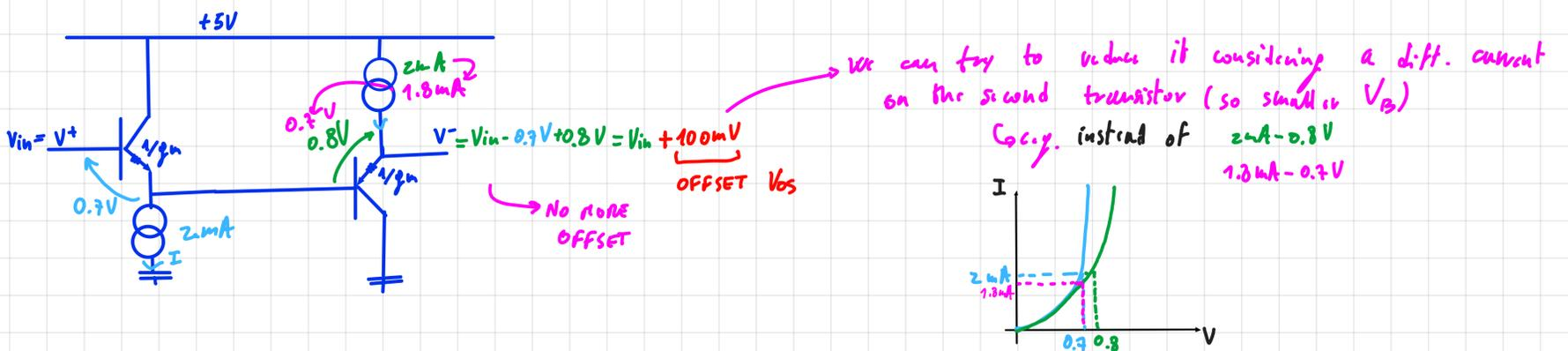
But in reality the transistor characteristics change also for temperature changes  $\rightarrow$  so we still have offsets!
