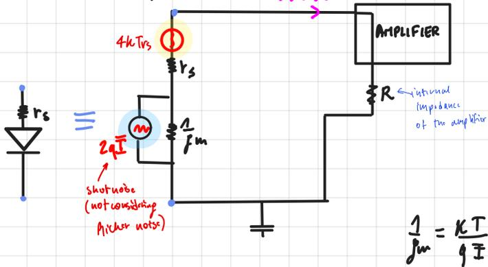
$$\frac{v_{noise}^2}{\Delta f} = 2qI \left( \frac{1}{g_m} \right)^2 \cdot R^2 + 4kT r_s \left( \frac{R}{R + r_s + \frac{1}{g_m}} \right)^2$$
