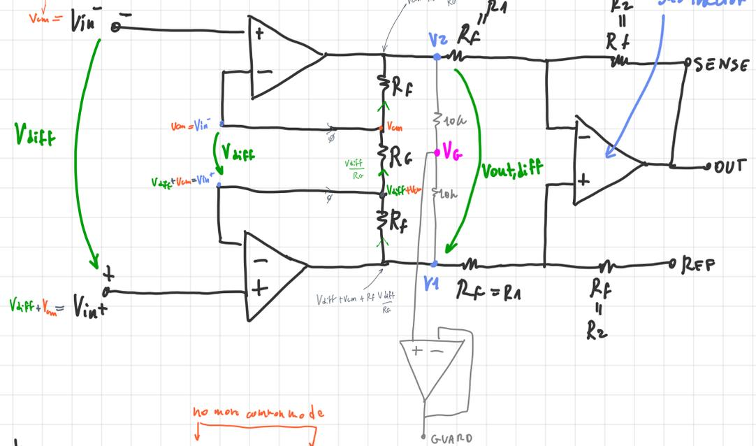
$$V_{out,diff} = V_{diff} + V_{cm} + R_f \frac{V_{diff}}{R_g} - V_{cm} + R_f \frac{V_{diff}}{R_g} = \left( \frac{V_{diff}}{R_g} \right) (R_f + R_g + R_f) = V_{diff} \left( 1 + \frac{2R_f}{R_g} \right)$$
