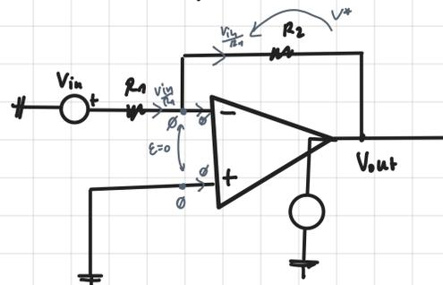
$V_{out} = -V^+ = -\frac{V_{in} R_2}{R_1}$
