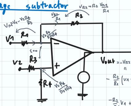
$$V_{out1} = -\frac{R_2}{R_1} V_1$$
