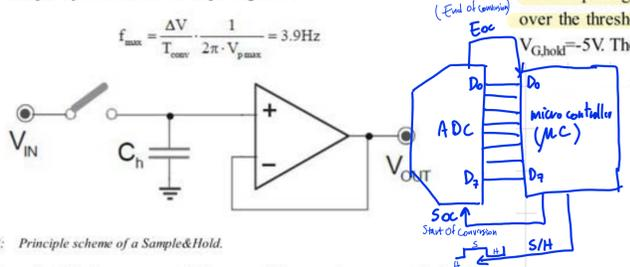
Fig. 6.28: Principle scheme of a Sample&Hold.
