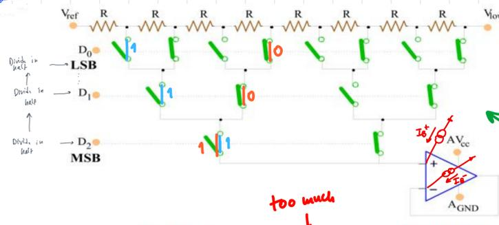
**Components:**  $2^n$  resistors and  $2^{n+1}$  pass-transistors (i.e.  $2^{n+2}$  MOSFETs)
