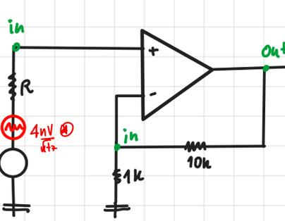
Fig. 1.10: Circuit for the equivalent noise bandwidth computation.
