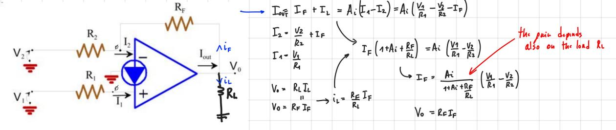
**Note:** If we don't want to connect any voltage to an input pin, let's put anyway a resistance, because due to the mismatches of the internal circuit there will be anyway a small volt. therefore a big cur.
