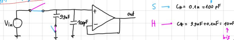
but this confg. has a problem since in the S phase the 9.9nF is disconnected it means it doesn't store basically no voltage, so when in H phase we close it on 9.9nF it will be a very small voltage on it.
