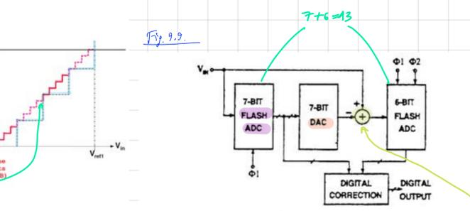
Example 12bit ADC: a flash ADC should require 4096 comparators the half-flash ADC instead needs  $2^7+2^6=192$  comparators (1bit overlap)
