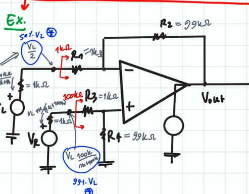
PROBLEM: If the  $V_1=V_2$  will have a voltage mismatch at the input.
