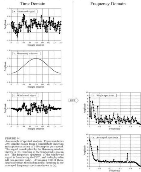
FIGURE 9-1 An example of spectral analysis. Figure (a) shows 256 samples taken from a (simulated) undersea microphone at a rate of 160 samples per second. This signal is multiplied by the Hamming window shown in (b), resulting in the windowed signal in (c). The frequency spectrum of the windowed signal is found using the DFT, and is displayed in (d) (magnitude only). Averaging 100 of these spectra reduces the random noise, resulting in the averaged frequency spectrum shown in (e).
