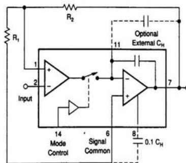
Wrong design (or drawing) this should be connect to ground
