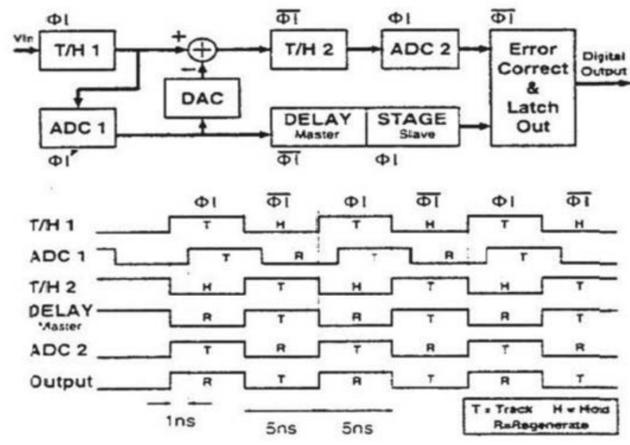
Fig. 9.20: Pipelined ADC timing graph.
