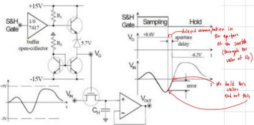
$$\Delta V_{aperture} = \frac{dV_{in}}{dt} \cdot T_{aperture} = 2\pi \cdot f_{max} \cdot V_{in,max} \cdot T_{aperture}$$
