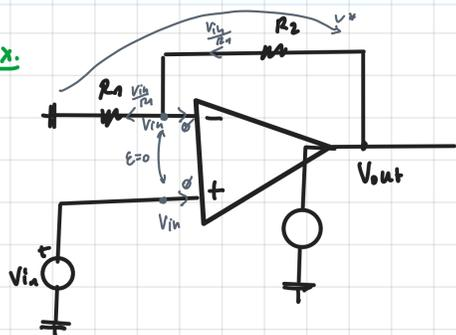
→  $V_{out} = V^+ = \frac{V_{in} (R_1 + R_2)}{R_1}$
