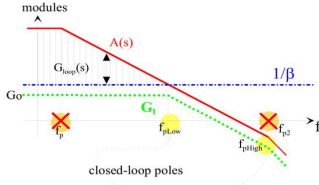
$$G_{I,real} = \frac{\tilde{A}}{1 + A \cdot \beta} = \frac{-\frac{R_2}{R_1 + R_2} \cdot A}{1 + A \cdot \beta} = \begin{cases} -\frac{R_2}{R_1} = -\frac{1}{\beta} \cdot \left(\frac{R_2}{R_1 + R_2}\right) & \text{if } 1/\beta \ll A \text{ (i.e. if } |G_{loop}| \gg 1) \\ -\left(\frac{R_2}{R_1 + R_2}\right) \cdot A & \text{if } 1/\beta \gg A \text{ (i.e. if } |G_{loop}| \ll 1) \end{cases}$$
