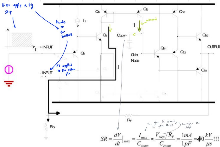
$$SR = \frac{dV}{dt} \Big|_{\max} = \frac{I_{\max}}{C_{\text{comp}}} \approx \frac{V_{\text{step}} / R_F}{C_{\text{comp}}} = \frac{1\text{mA}}{1\text{pF}} = 10 \frac{\text{kV}}{\mu\text{s}} !!!$$
