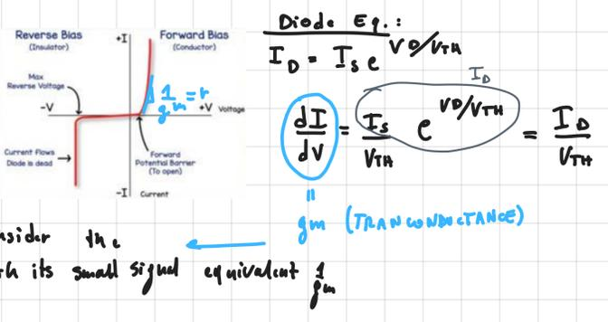
We can consider the diode with its small signal equivalent of  $\frac{1}{g_m}$
