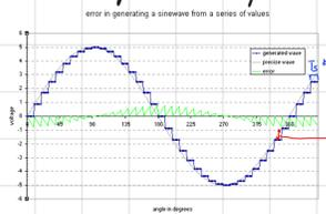
If INL is very low it means that the quantization error will be at most  $\pm \frac{LSB}{2}$  (hardly)
