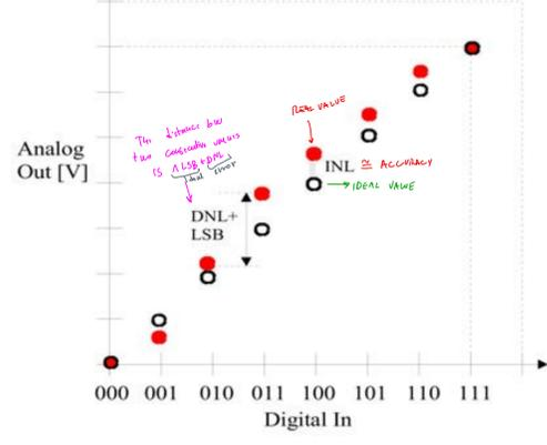
**Offset:** output when input is 000 } can be fixed
