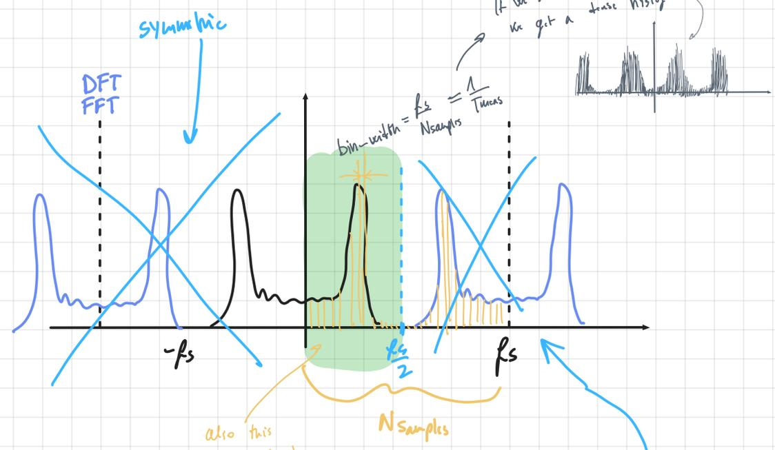
If the signal is real the spectrum is symmetric also around  $\frac{f_s}{2}$ . We study the spectrum just in this area  $\in [0, \frac{f_s}{2}]$ .
