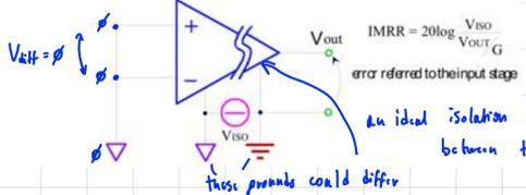
an ideal isolation is when, even if there's a difference between the two grounds (or biases),  $V_{out} = 0$
