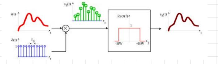
Generally, the sampling operation relies on a circuit named *Sample&Hold* (described in detail in this chapter), which does not generate analog pulse samples, but periodically picks the signal setting the amplitude at the output for a period  $T_s$ , as shown in Fig. 6.5.
