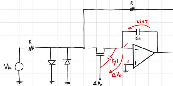
$V_{inj} = \Delta V_G \frac{C_{pd}}{C_H}$
