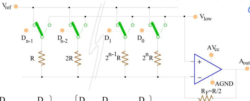
$$V_{out} = V_{ref} \frac{R_f}{R} \left\{ \frac{D_{n-1}}{1} + \frac{D_{n-2}}{2} + \dots + \frac{D_0}{2^{n-1}} \right\} = V_{ref} \left\{ \frac{D_{n-1}}{2} + \frac{D_{n-2}}{2^2} + \dots + \frac{D_0}{2^n} \right\}$$
