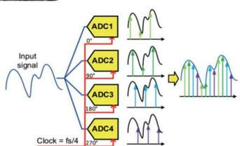
Components: • ADCs → put in parallel
