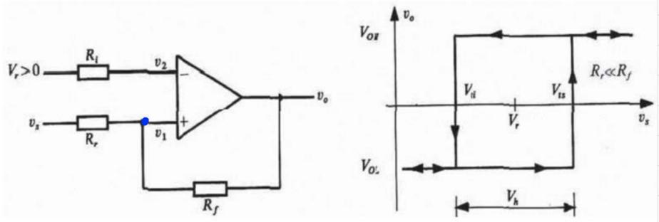
The non-inverting Schmitt Trigger is similar to the inverting configuration, but the input signal  $v_s$  and the reference  $V_r$  are reversed, as shown in Fig. 2.51. With an analogous reasoning, as for the inverting configuration, we have:
