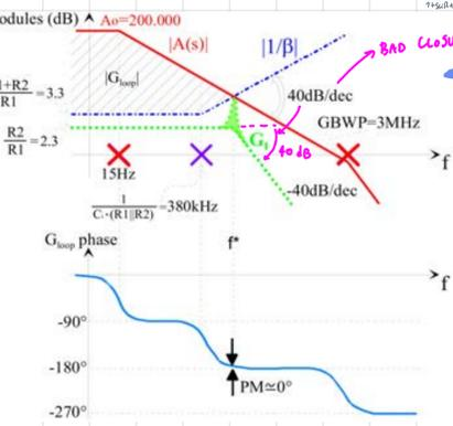
Note For  $\frac{1}{\beta}$  we can have different characteristic based on the values of  $C_i$  and  $C_c$  (or  $C_f$ ):
