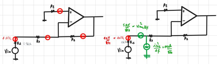
$$R_{Sopt} = \sqrt{\frac{(5\text{ nV}/\sqrt{\text{Hz}})^2}{(10\text{ pA}/\sqrt{\text{Hz}})^2}} = \frac{5\text{ nV}/\sqrt{\text{Hz}}}{10\text{ pA}/\sqrt{\text{Hz}}} = 500\text{ }\Omega$$
