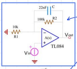
Let us study the frequency response of the non-inverting configuration with a capacitor on the feedback network (approximate integrator) which is shown in Fig. 3.26. If we want to calculate the forward block  $\tilde{A}$ , "turn off" the feedback (Fig. 3.27) and compute:
