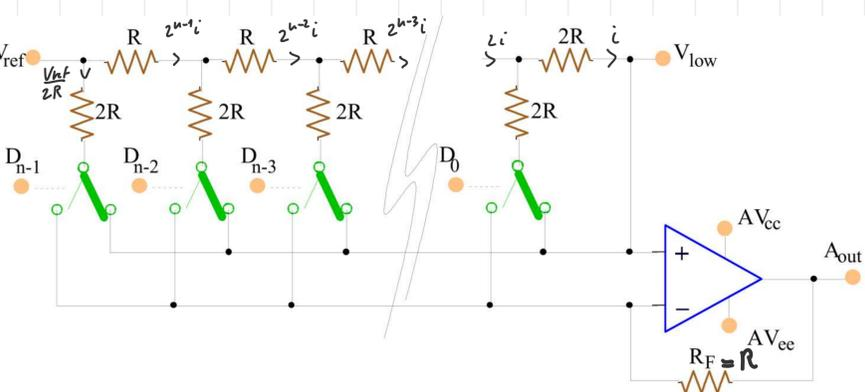
**Components:** •  $3n$  resistors → current divider
