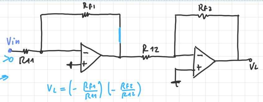
$$V_L = \left(-\frac{R_{f1}}{R_{f1}}\right) \left(-\frac{R_{f2}}{R_{f2}}\right) V_{in}$$
