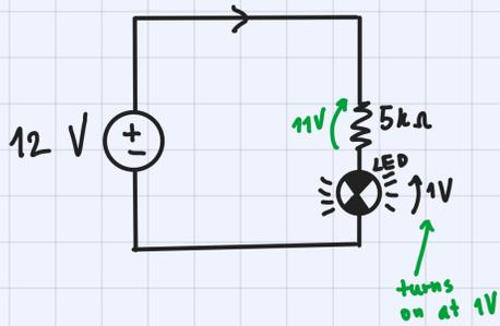
The LED turns ON at 1V, meaning we want on the resistor a 11V voltage drop.
