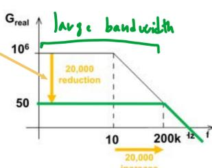
For example:  $F=1/50$   $G_{loop} = -20,000$   $G_{real} = 50$   $\text{pole} = 200,000 \text{ Hz}!$
