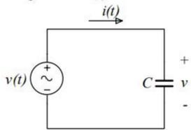
Figure 3. Fundamental capacitor circuit
