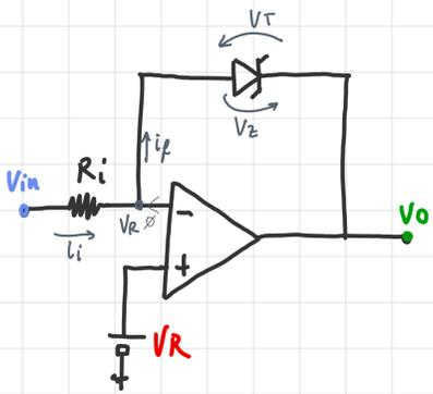
$$i_f = i_i = \frac{V_{in} - V_R}{R_i}$$
