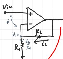
$$i_L = \frac{V_{in}}{R_1}$$
