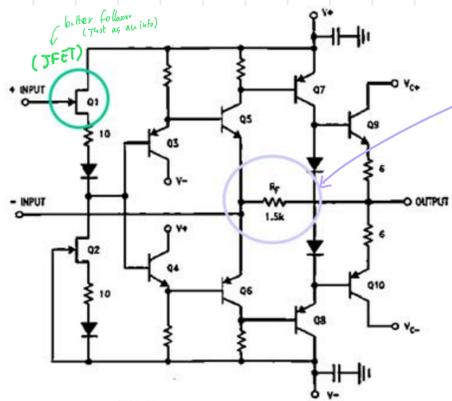
Some manufacturers put  $R_f$  directly inside, because we don't change it anyway (const. pole property of CFA for low gain) ↳ 'cause if we want to change the gain we change  $R_G$
