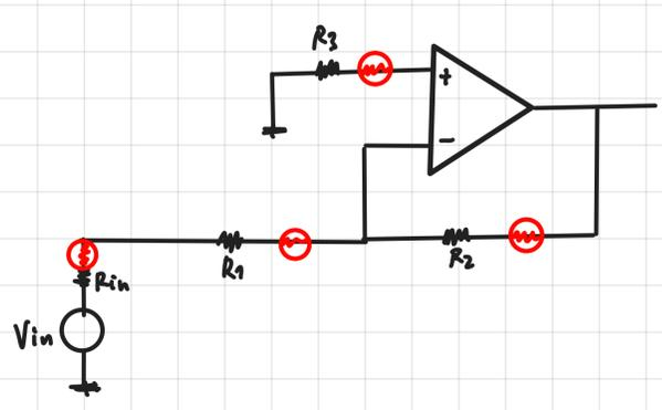
$$NF = \frac{SNR_{in}}{SNR_{out}} = \frac{S_{in}}{N_{in}} \cdot \frac{N_{out}}{S_{out}} = \frac{N_{out}}{N_{in} \cdot G} = \frac{\text{tot. out. noise}}{\text{out. noise due to just } R_{in}}$$
