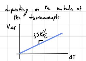
A possible explanation of the flicker noise  $\frac{1}{f}$  comes from the thermocouples formed at the pins that usually have a noise trend of  $\frac{1}{f}$
