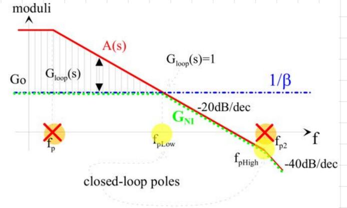
Phase Margin:  $\Phi_M = 180^\circ - 90^\circ - \arctg \left| \frac{f_{pLow}}{f_{p2}} \right|$
