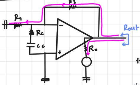
$$R_{out}(0) = \frac{R_{stupid}}{1 - G_{loop}} = \frac{(R_1 + R_2) \parallel R_o}{1 + A_o \cdot \frac{R_1}{R_1 + R_2 + R_o}}$$
