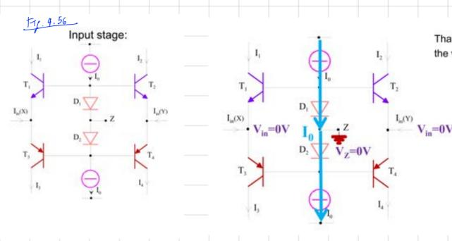
Thanks to pin Z the voltage at the inputs is set
