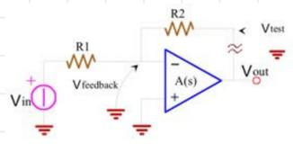
$$\beta = \frac{V_{feedback}}{V_{test}} = \frac{R_1}{R_1 + R_2}$$
