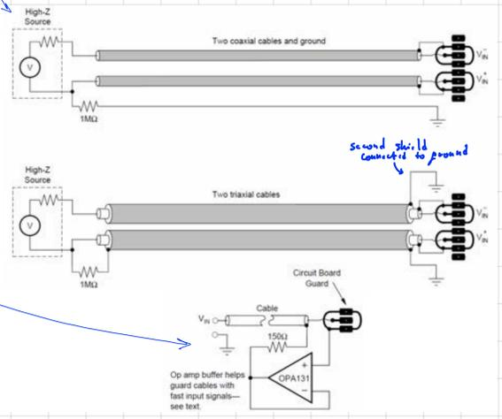
In the INA110, whose datasheet is attached below, it is possible to choose between x10, x100, x200, and x500 gains. The Guard connection (to drive the signal coaxial cable) is not present in the INA110. It is possible to put it externally, as shown in the figure of the data-sheet of the INA110 at the end of the chapter.
