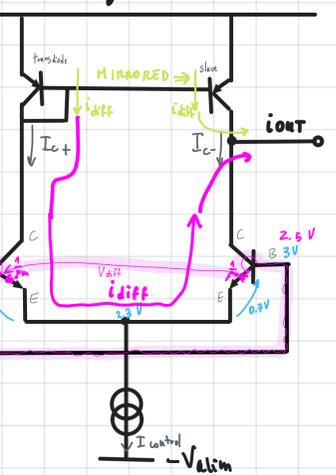
$$i_{out} = 2 i_{diff} = \frac{2 \cdot V_{diff}}{2 \cdot \frac{1}{f_{in}}} = G_m V_{diff}$$
