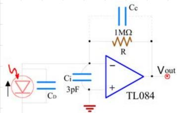
There are various types of amplifiers for photodiodes: some of them read the tension that builds up between their terminals and amplify it whereas others read the currents flowing and transform these currents into tension. The drawback of the former, if realized with active circuitry, is that part of the signal is lost in stray components of the circuit. The quality of the latter, instead, is that the current signal is injected into the virtual ground and therefore is not lost.
