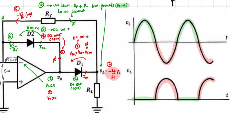
Remember that for diode to be ON at least  $V_T = 0.6V$  is required across the diode.
