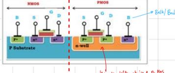
But introduces a parasitic diode/inverse bias (no problem when using MOS as an amplifier because  $V_D > V_S \rightarrow$  diode OFF)
