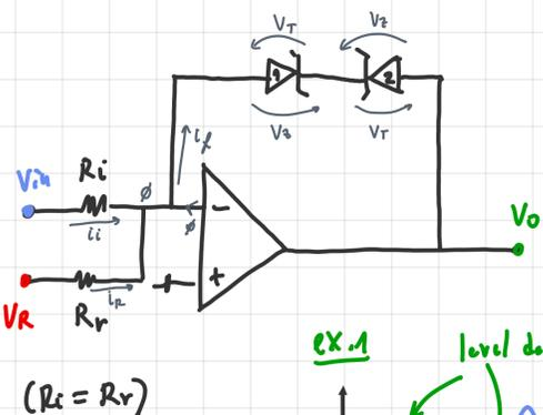
$$i_f = i_1 + i_2 = \frac{V_{in}}{R_i} + \frac{V_o}{R_r}$$
