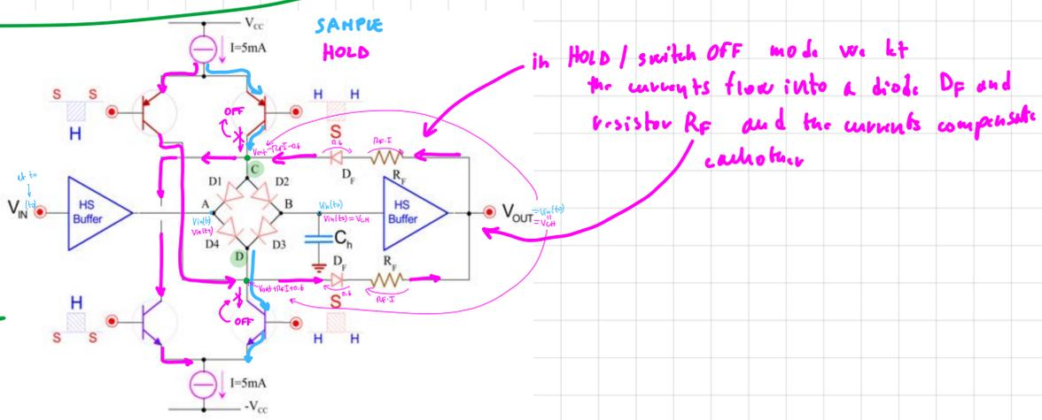
in HOLD / switch OFF mode we let the currents flow into a diode Df and resistor Rf and the currents compensate each other
