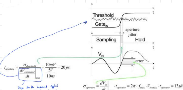
$$t_{aperture} = \frac{\sigma_{threshold}}{\frac{dV_{command}}{dt}} = \frac{10mV}{\frac{5V}{10ns}} = 20ps$$
