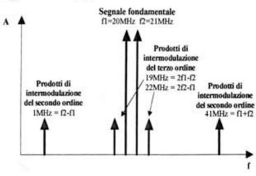
InterModulation Distortion: ratio among all intermodulation products and 2 useful signals
