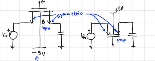
in such way that we reverse bias both the diode forming bulk and the one bulk and drain so parasitic diodes OFF
