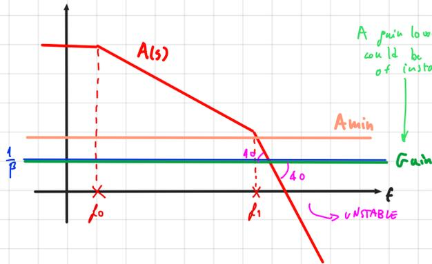
A gain lower than  $A_{min}$  could be the source of instability
