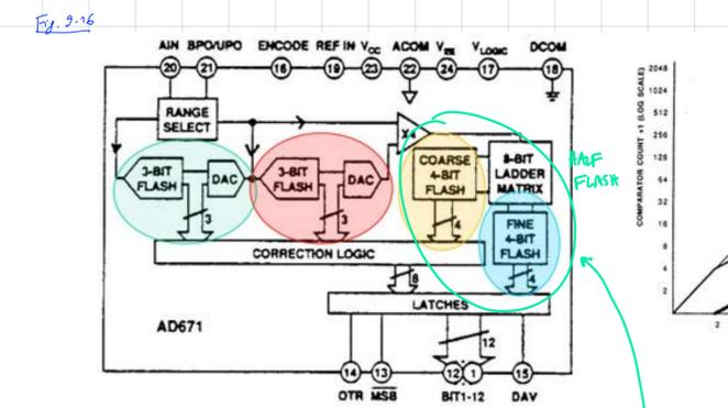
Example of a 4-step ADC: First 3bit and second 3bit flash ADCs, then first 4bit and second 4bit half-flash Overall just 48 comparators!
