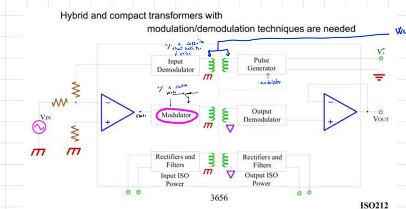
We can isolate 2 parts through the magnetic effect of the transformers
