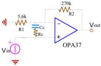
$R_c, C_c$  are bootstrapped on the input signal, hence they have no role in the circuit (what's up here then?!)
