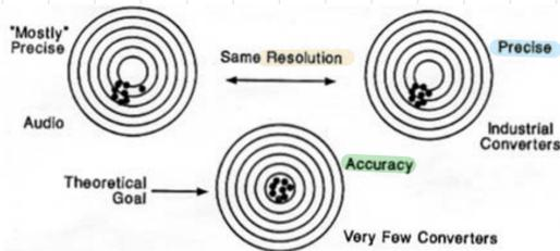
**Resolution** subdivision of output dynamics that the converter is able to resolve
