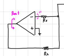
$R_{out} = \frac{(R_1 + \infty) \parallel R_2}{1 - G_{loop}} = \frac{R_2}{1 - G_{loop}} = \frac{R_2}{1 + A_0}$
