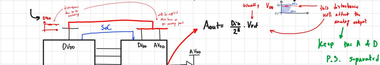
connect them as close as possible to the battery in this way any demand of currents (due to possible R or L) that will cause big voltage drops
