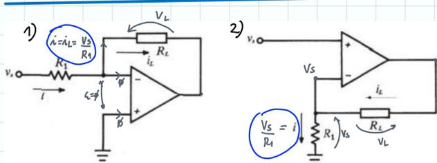
Issues: • If  $R_1 \uparrow$  Gain:  $\frac{i_{out}}{V_{in}} = \frac{1}{R_1} \downarrow$
