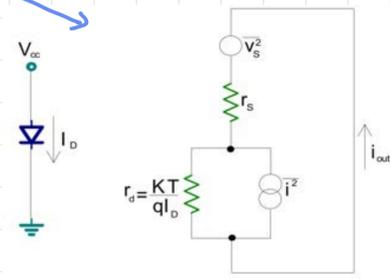
Can be modeled as a thermal noise on an eq. resistor
