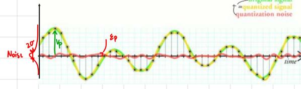
In particular:  $SNR_{\text{ideal}}$  (just considering quantization noise):  $SNR_{\text{ideal}} = SNR_{\text{max}} = \frac{S_{\text{max}}}{N_{\text{min}}} = \frac{\left(\frac{FSR}{2\sqrt{2}}\right)^2}{\frac{FSR^2}{12 \cdot 2^{2n}}} = \frac{12 \cdot 2^{2n}}{4 \cdot 2} = \frac{3}{2} 2^{2n}$
