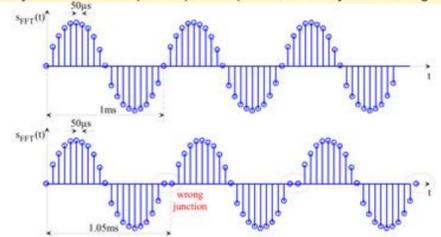
To increase the frequency resolution (i.e. the number of histograms in the FFT), it is possible to increase the number  $N$  of collected data. Fig. 6.24 and Fig. 6.25 show the processing of the previous sinusoid, which was performed with a higher number of samples, with  $N=200$  and  $N=256$ , respectively, corresponding to the total measurement duration of  $N \cdot T_s = 10\text{ms}$  and  $12.8\text{ms}$ , respectively, with the same sampling frequency.
