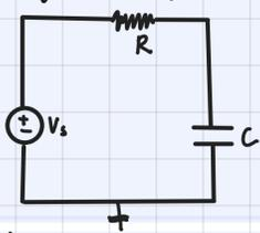
The capacitor **DOESN'T** dissipate power  $\rightarrow$  It just charges and discharges (reactive component)
