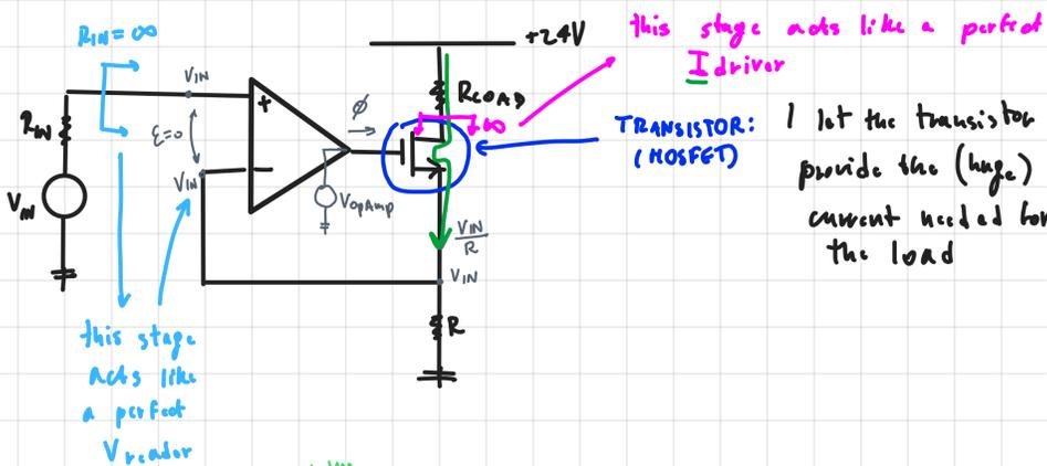
→ the OpAmp can provide no current but just a voltage, we'll have the current  $\frac{V_{in}}{R}$  flowing through the transistor instead of directly the OpAmp
