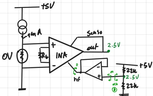
↳ In this case considering that inside the INA there will be the resistors that must see a voltage source (so with  $\square$  instead of  $\square$ )
