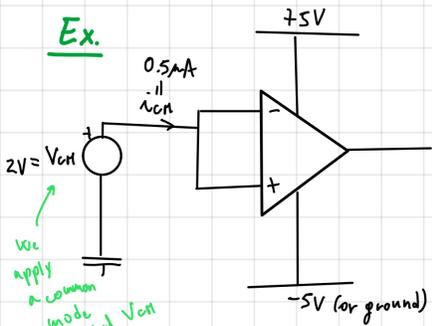
→ If we measure a current it means there's an input impedance
