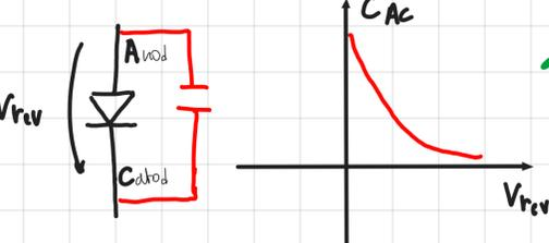
we reduce the parasitic capacitances now at points C and D we have a higher voltage → D2 and D4 go into reverse too
