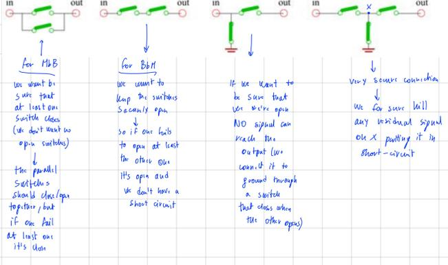
For BbM we want to be sure that at least one switch close (we don't want to open switches) the parallel switches should close together, but if one fails at least one it's done
