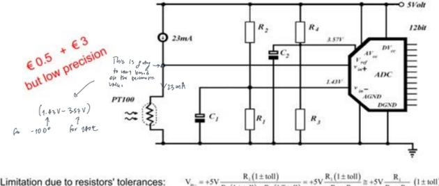
Limitation due to resistors' tolerances:  $V_{in} = +5V \cdot \frac{R_1(1 \pm \text{tol})}{R_1(1 \pm \text{tol}) + R_2(1 \mp \text{tol})} = +5V \cdot \frac{R_1(1 \pm \text{tol})}{R_1 + R_2}$
